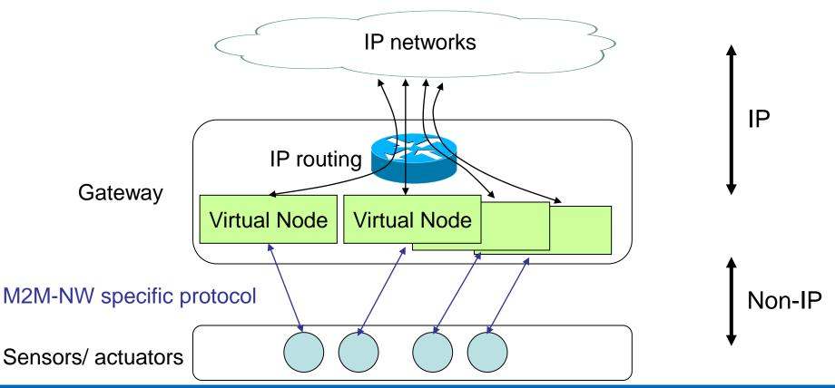
Modeling IP-based M2M-NW
